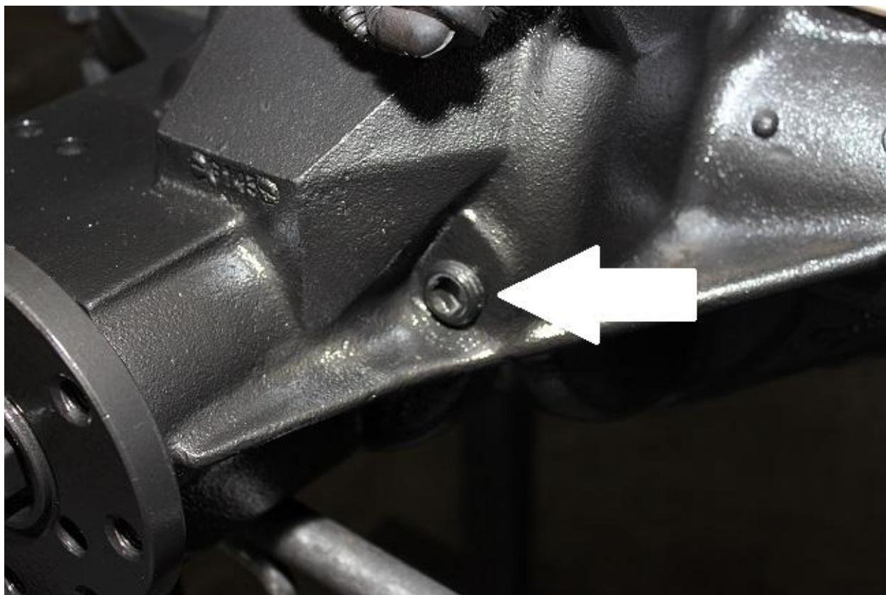
**Failure to fill from this location will cause over-filling of the differential and possible damage to the axle and void warranty!! Or pending pinion angle, under filling of the axle. All ford 8.8 axles should have 2.85-3 quarts. If you have a pinion angle above 15 degrees 3.5 quarts is recommended however it may release some fluid out of the breather.**
