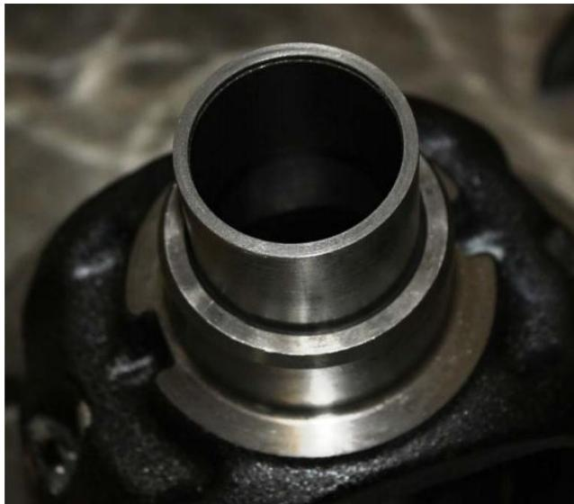
B. Install bushing flush with carrier (Be careful not to drive the bushing past flush as the design of the bushing is longer than the stock needle bearing to provide more support, however if driven to much past flush it will contact the spider gear)
