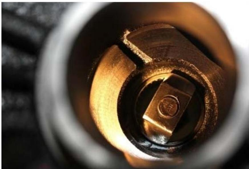
G. REMOVE THE PAPERTOWEL OR STOP INSTALLED INTO SPIDER GEAR!!!!
