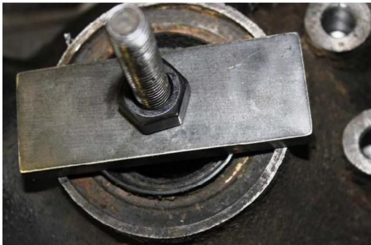
E. Hand tighten nut to plate, and insure that tool is centered.
