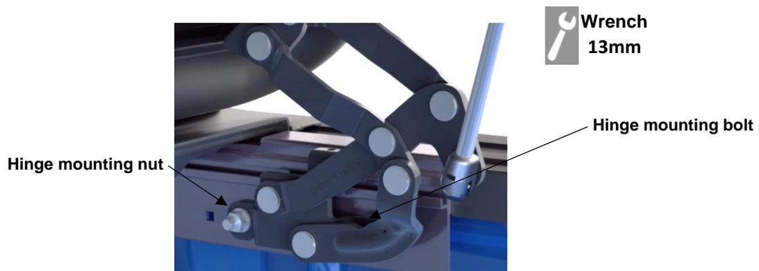
4. Have your friend carefully lower the cover until the hinge bracket alignment tabs rest on the bedrail channel. This will support the cover while you and your associate move to the sides of the truck.
