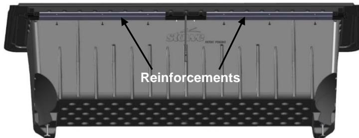
Install the six (6) attachments screws to secure the rear flange reinforcements to the underside of the tool box flange. The screws will thread into the mounting clips installed in the flange.
