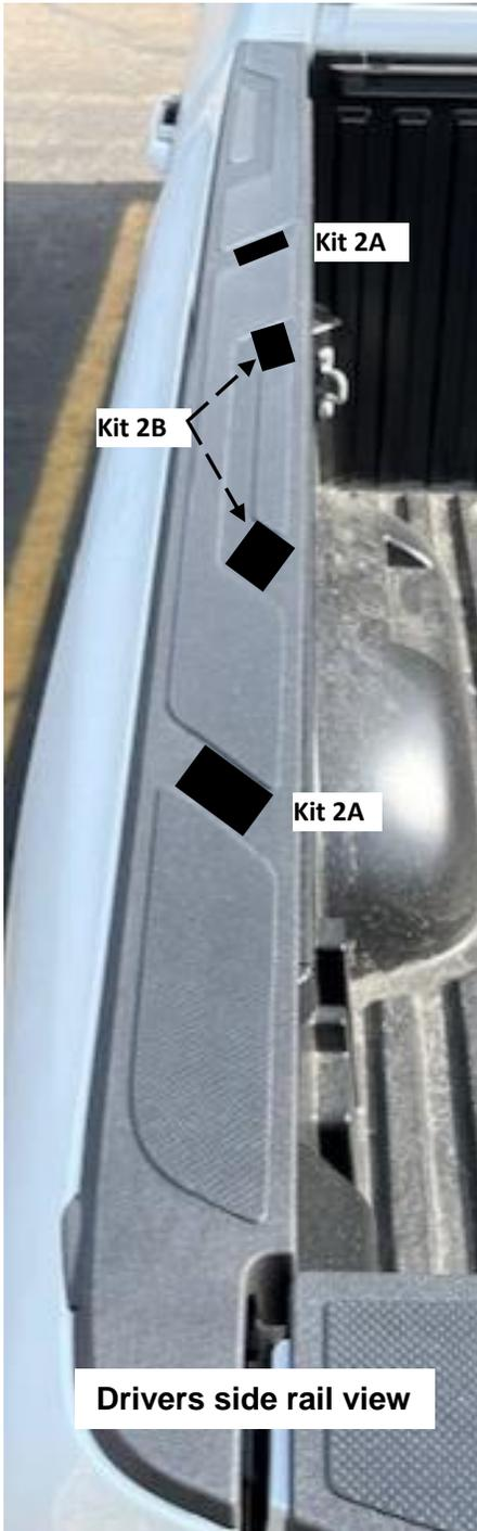
Clean the rib gaps with rubbing alcohol before applying the fillers in the locations shown below.
