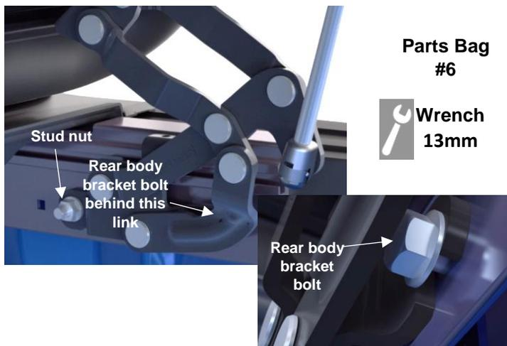
Install and hand tighten only, the stud nut on both sides of the truck.
