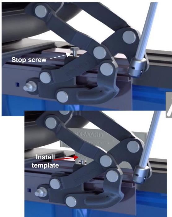
**Parts Bag #6** Install the rear hinge stop screw and set the installed height using the cutout in the bed rail installation template as an initial guide.
