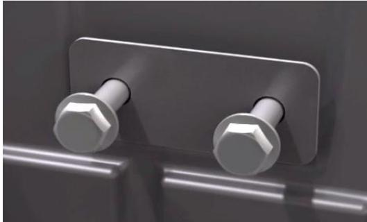
**Parts Bag #5** Hand start and then remove all four hinge bolts to ensure proper alignment between the spacer and the bed rail.
