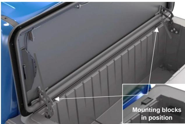
**Parts Bag #5** Place the front cover mounting blocks in the pockets on either side of the compartment front flange.
