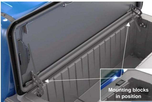
**Parts Bag #3** Place the front cover mounting blocks in the pockets on either side of the compartment front flange.
