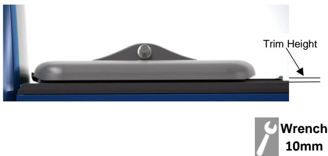
Re-position the striker vertically as required to adjust the trim height of the cover along the side of the truck while maintaining the latching function to the striker. The trim height should be about even from front to rear looking at the cover on the driver's side.
