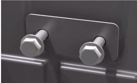
**Parts Bag #3** Hand start and then remove all four hinge bolts to ensure proper alignment between the spacer and the bed rail.
